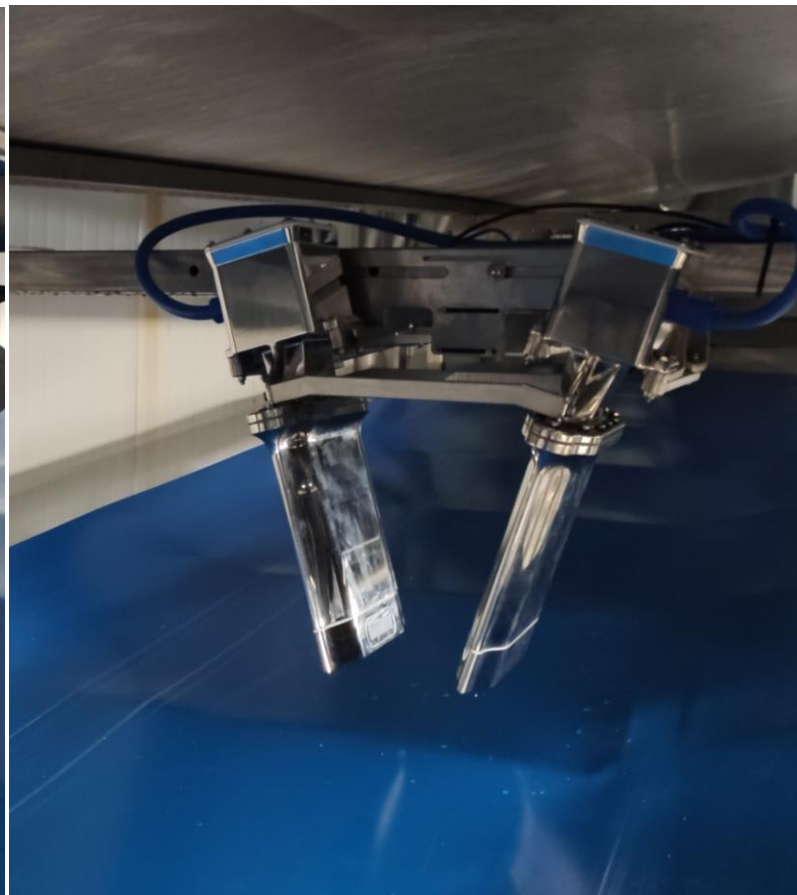
Figure 1: Installed Moisture-Sense sensor - Single Plow version (left) and Double Plow version (right).
